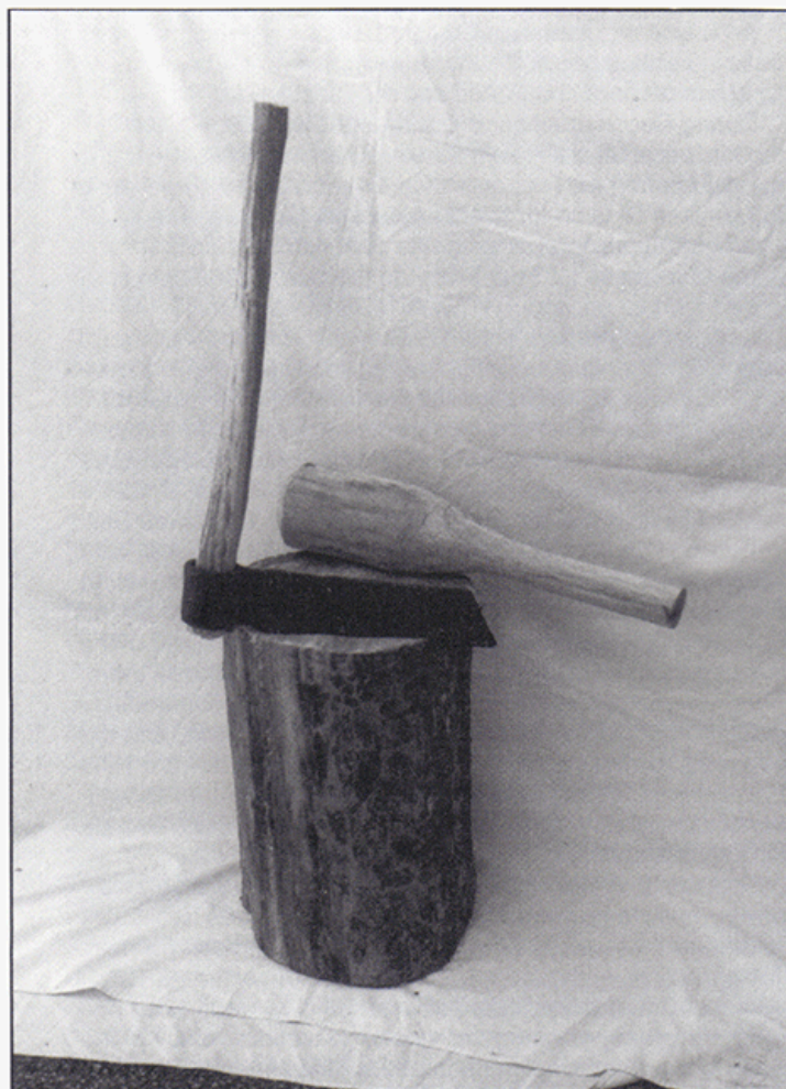
Froe, shingle bolt, and one-piece maul (from live oak).
