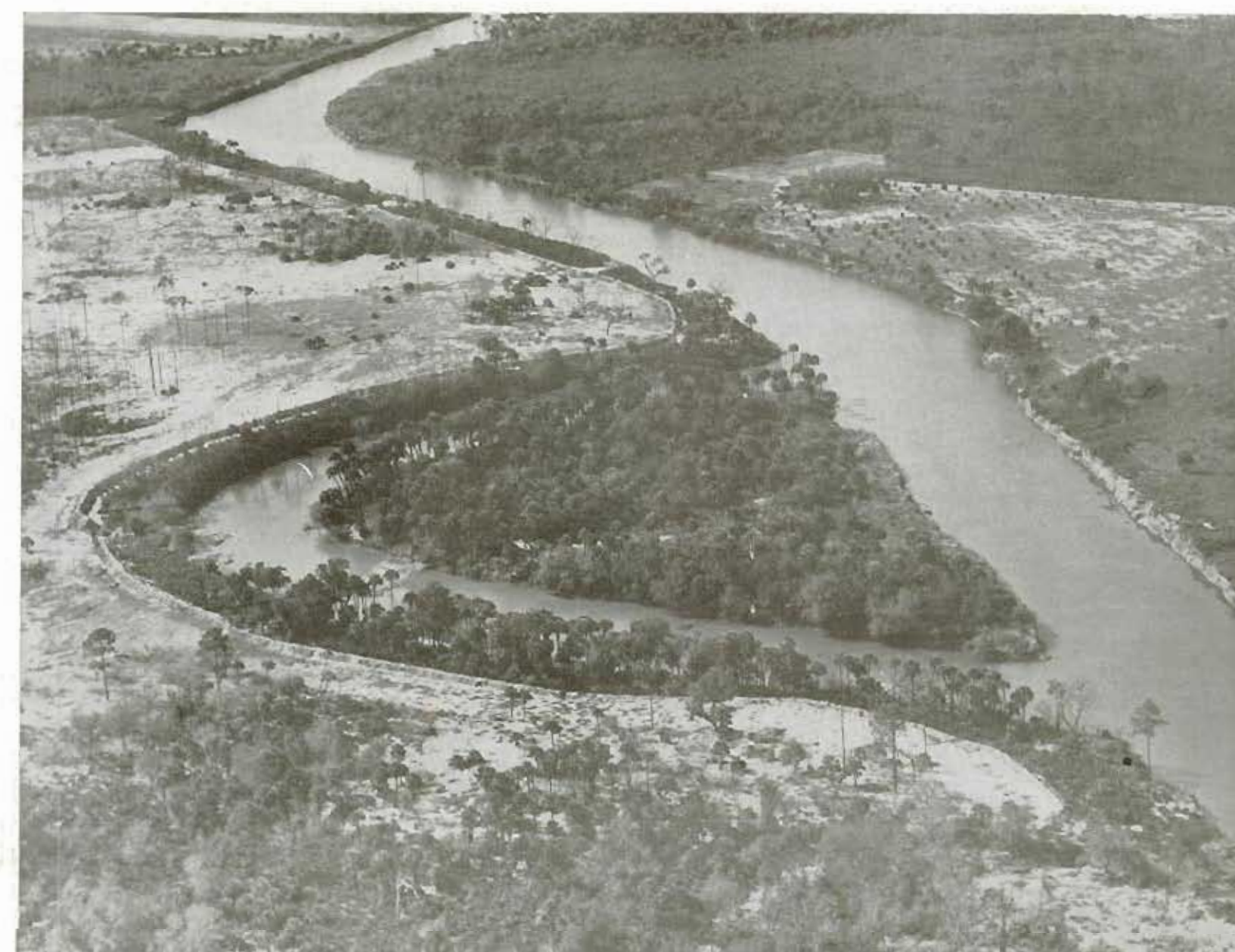
This Picture Shows One of the Many Horseshoe Bends in the Caloosahatchee River Which Have Been Eliminated by the Fed- eral Government in the $1,500,000 Deepening and Straightening Operation On The Moorehaven-Fort Myers Link.
