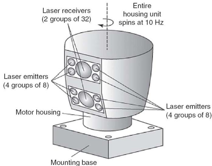
**Figure 2.** Velodyne scanner (Courtesy of M. Shand).
